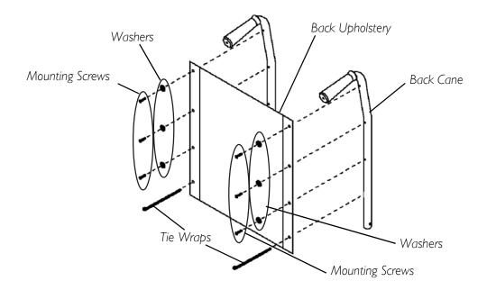
FIGURE 8.2 Replacing the Back Upholstery
